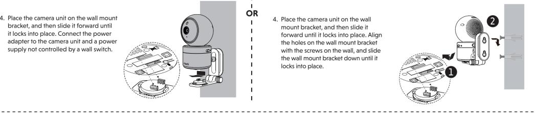
5. You can maximize your camera unit's viewing angles by tilting the wall mount bracket. Hold the camera unit, and then rotate the knob in anticlockwise direction. This will loosen the joint of the wall mount bracket. Tilt your camera unit up or down to adjust to your preferred angle. Then, rotate the knob in clockwise direction to tighten the joint and secure the angle.
