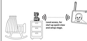
You may experience reduced signal strength if your parent unit and baby unit are far apart, or there are obstructing factors, such as internal walls, between them. You have to set up **Router mode** to connect the units via your home Wi-Fi network to improve the connection between your parent unit and baby unit.
