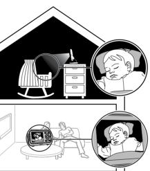
The baby unit has infrared LEDs that allow you to see your baby clearly at night or in a dark room. When the baby unit detects low light levels, the infrared LEDs are switched on automatically. The images from the baby unit are in black and white, and 🥨 appears on the parent unit screen.
