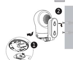
4. Place the baby unit on the wall mount bracket, and then slide it forward until it locks into place. Align the holes on the wall mount bracket with the screws on the wall, and slide the wall mount bracket down until it
