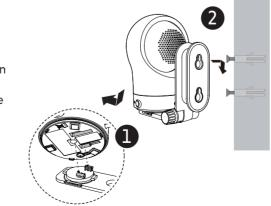
5. You can maximise your baby unit's viewing angles by tilting the wall mount bracket. Hold the baby unit, and then rotate the knob in an anticlockwise direction. This will loosen the joint of the wall mount bracket. Tilt your baby unit up or down to adjust to your preferred angle. Then, rotate the knob in a clockwise direction to tighten the joint and secure the angle.
