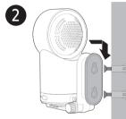
5. You can maximise your baby unit's viewing angles by tilting the wall mount bracket. Hold the baby unit, and then rotate the knob in an anticlockwise direction. This will loosen the joint of the wall mount bracket. Tilt your baby unit up or down to adjust to your preferred angle. Then, rotate the knob in a clockwise direction to tighten the joint and secure the angle.
