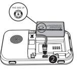
• Make sure the label THIS SIDE UP is facing up while inserting the battery
