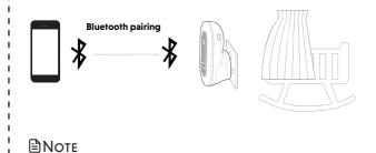
After the soother enters the Bluetooth pairing mode, the blue light on the soother will continue to fade in and out until it is connected to a device.
