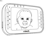
If both units are not connected, the parent unit displays No link to CAM 1 and Linking... on the screen. The LINK light first flashes and then turns off. Move the parent unit closer to the baby unit.
