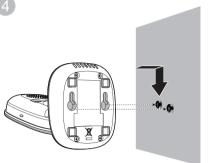
baby unit with the screws on the wall. Slide the baby unit down until it locks into place.
