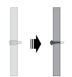
Insert the screws into the holes and tighten the screws until only 6.5 mm of the screws are exposed.
