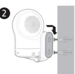
5. You can maximise your Baby Unit viewing angle by tilting the wall mount bracket. Hold the Baby Unit, and then rotate the knob in an anticlockwise direction. This will loosen the joint of the wall mount bracket. Tilt your Baby Unit up or down to adjust to your preferred angle. Then, rotate the knob in a clockwise direction to tighten the joint and secure the angle.
