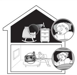
The baby unit has infrared LEDs that allow you to see your baby clearly at night or in a dark room. When the baby unit being viewed detects low light levels, the infrared LEDs are switched on automatically. The images from the baby unit are in black and white, and 2 appears on the screen.
