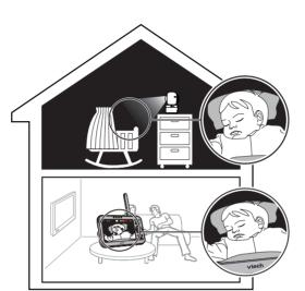
The baby unit has infrared LEDs that allow you to see your baby clearly at night or in a dark room. When the baby unit being viewed detects low light levels, the infrared LEDs are switched on automatically. The images from the baby unit are in black and white, and appears on the screen.
